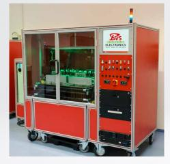
At the **test stands** developed in-house, the functionality of power components is tested under realistic conditions using solar field
